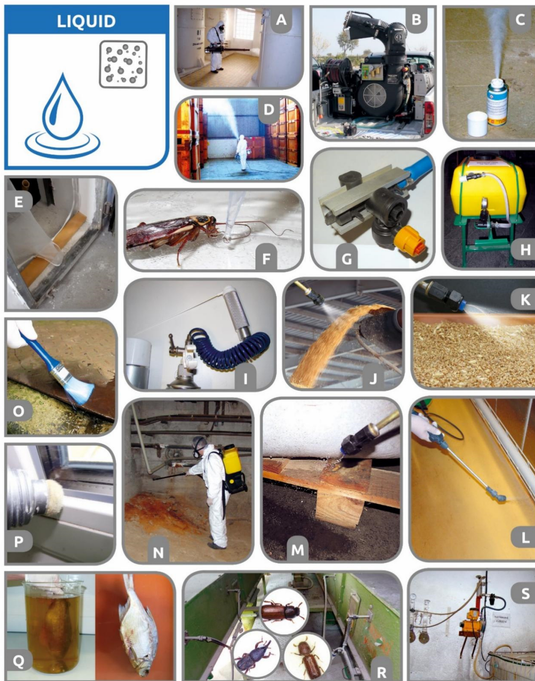
Figure 3. Liquids (A) Portable aerosol thermal fogging in food industry silos; (B) vehicle-carried cold aerosol applicator; (C) cold aerosol container pressurized with propellant; (D) cold ULV aerosol application in a store; (E) barrier treatment—fluid insecticide-soaked sponge door mat; (F) baits—fluid carrier with attractant toxicant or genetic disruptor (dsRNA encapsulated with liposome carriers); (G) spray nozzle with device for its attachment to grain conveyor belts; (H) mobile compressor and sprayer for grain protectant application; (I) dual injection spray/aerosol device; (J) visualization of spray protectant applied on grain moving on a conveyor belt; (K) visualization of spray/aerosol protectant application on falling grain; (L) band barrier or spot spray treatment; (M) spray barrier treatment of transport pallets; (N) broadcast spray of walls; (O) insecticide brushing; (P) insecticide sponging; (Q) dip application of insecticide protectant on the surface of dried fish; (R) multipoint treatment of grain moving on covered conveyor belts (piping is visible; spray nozzles hidden inside covered equipment); (S) wall-mounted compressor, insecticide tank, and piping for grain treatment located at the bottom of a grain silo (photographs (A–S): V. Stejskal; R. Aulicky, T. Vendl).
