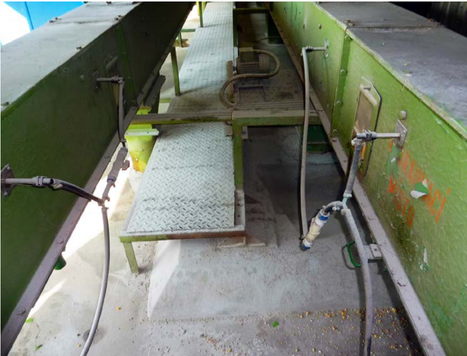
Residual insecticide sprays (so called grain protectants) are mostly based on pyrethroids. They are commonly applied on grain during its transport on conveyer belts.
